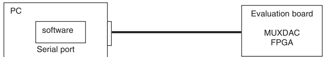
Figure 4-7. User Interface Hardware Implementation
