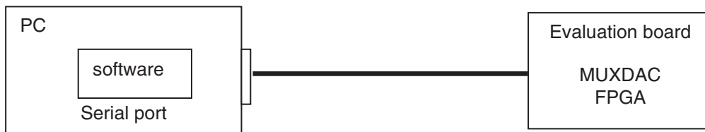
Figure 4-7. User Interface Hardware Implementation
