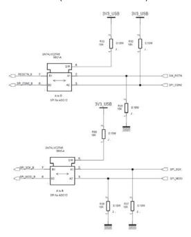
Figure 7-7. Electrical Schematics (Output Connectors Ports A and B)
