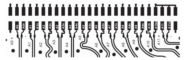
Figure 5-16. Differential Digital Outputs 2.54 mm Pitch Connector (Port B)
