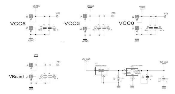
Figure 7-2. Power Supplies Decoupling
