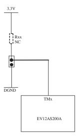
■ The default setting for RS, TM and MODE\_n is when their respective jumper is OUT.
