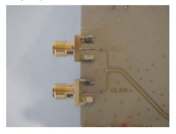
The jitter performance on the clock is crucial to obtain optimum performance from the ADC. We thus recommend to use a very low phase noise clock and to filter the clock signal if a fixed frequency is used.
