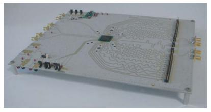
The board dimensions are 260 mm x 210 mm. The board comes fully assembled and tested, with the EV12AS200A installed.
