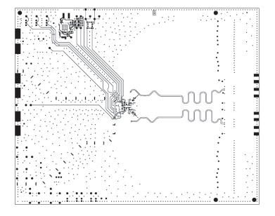
Figure 7-10. AGND, DGND (Separate Planes) LAYER 2 & 5
