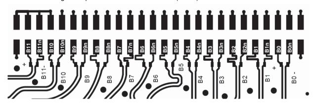
Figure 5-17. Differential Digital Outputs 2.54 mm Pitch Connector (DR, DRN Signal)
