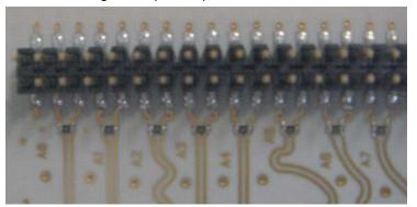
Double row 2.54 mm pitch connectors are used for the digital output data. The lower row is connected to the signal while the upper row is connected to Ground.
