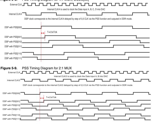
Figure 5-8.PSS Timing Diagram for 4:1 MUX, OCDS[00]
