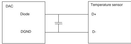
In characterization measurement a current of 1 mA is applied on the DIODE pin. The voltage across the DIODE pin and the DGND pin gives the junction temperature using the intrinsic diode characteristics below Figure 5-17 on page 27.
