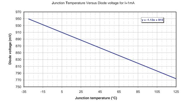
Figure 5-17. Diode Characteristics for Die Junction Monitoring
