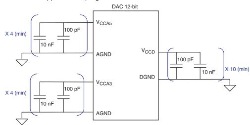
Figure 7-11. Power Supplies Decoupling Scheme
